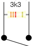
Normally Open devices do not allow current to flow through them until they are triggered, therefore the 3k3 resistors must be placed in parallel to the device as show.
