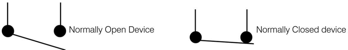
**Normally Closed:** Is when a devices output will allow current to flow through it, I.e. Like when a light switch is on and the globe is on and lighting up the room.
