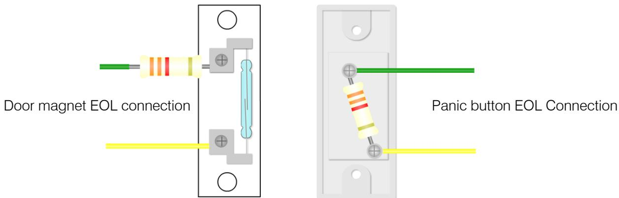
The Arm Zone is used to connect a device that will close momentarily to remove the 3k3 resistor from the zone for a second and return it back into the circuit. When the alarm panel sees this it will toggle the state of the alarm panel.
