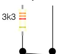
Normally closed device allows current to flow trough it until it is triggered, therefore the resistor must be placed in series with the device as shown.
