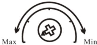
Adjust the response time of the receiver generating an alarm based on the time needed for an intruder to cross the beam area.
